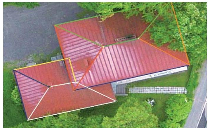
*Planar surfaces of roofs can be detected from laser points. Their edges can be edited only manual by using 'bird-eye view' and raw images as reference.*
